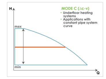
This mode is suitable for all underfloor heating systems, where all circuits must be balanced for the same drop in the head or for applications with no changeable pipe system curve (e.g. system without thermostatic valves).
