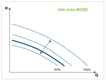
**Askoll E-PURE** features fixed speed operating curves by positioning the regulator at any point between the Min and Max positions; as a result it is possible to meet any installation requirements (from the single pipe, to the most modern and sophisticated systems) and ensure optimum performance.
