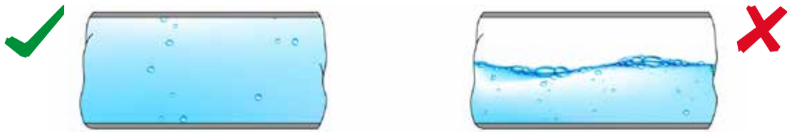
Fig. 5 The pipe must always be completely full of liquid
