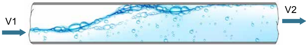
Fig. 37 Air pockets inside the pipe
