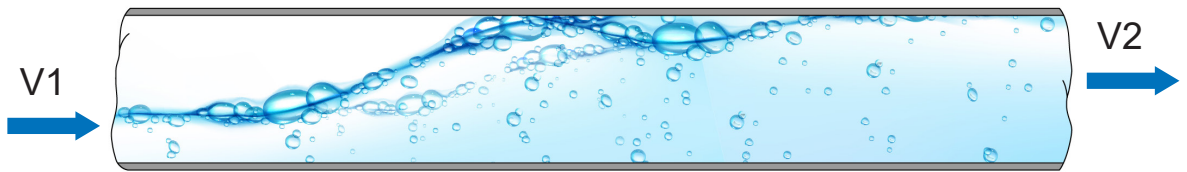
Fig. 31 Air pockets inside the pipe
